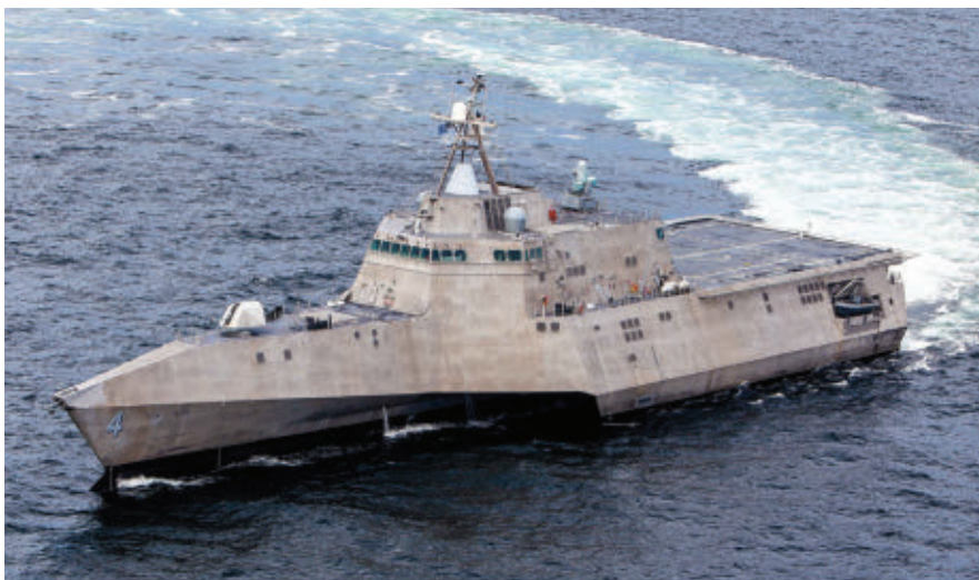
The Independence class LCS variant is on a trimarin hull. Shown here: the second trimarin, Coronado (LCS 4) underway after completing acceptance testing last fall.
